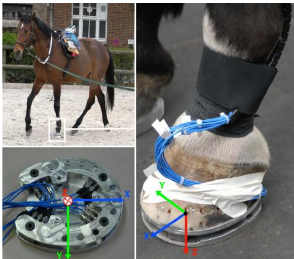
Figure 5. A force shoe described by Chateau et al. for use with horses [2].
