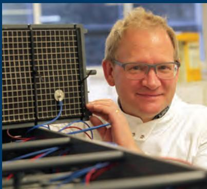
*Prof Tom Curtis with a Microbial Electrolysis Cell. Trialled with NWG, the cell produces valuable hydrogen gas, a source of clean energy, from raw sewage at ambient temperature.*
