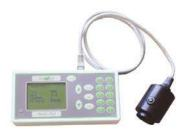
The Handy PEA chlorophyll fluorimeter consists of a compact, light-weight control unit encapsulating sophisticated electronics providing the high time resolution essential in performing measurements of fast chlorophyll fluorescence induction kinetics.
