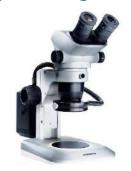
The stereo microscopes are an important asset in terms of monitoring samples and selecting materials or processing. For example, they can be used for visually checking for disease or the physical state of plant organs and tissues prior to downstream analysis. These observations are important to ensure that selection of materials is as consistent as possible.
