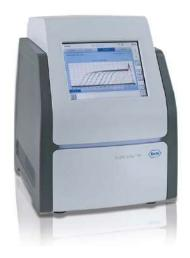
The qPCR (Light Cycler) and associated equipment (Qiacube and Nanodrop) are for the amplification and quantification of DNA/RNA using real-time or quantitative PCR. Examples could be monitoring the up or down regulation of transcripts or the detection and quantification of pathogens in plants or soils. The key advantage of qPCR is that it is a highly sensitive and specific, closed-tube, real-time system for the accurate detection and quantification of DNA targets.
