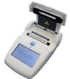
Genie III is a hand held, battery powered DNA amplification device for running Loop mediated AMPlification (LAMP) assays. LAMP, like PCR enables sensitive and specific amplification of target genes in hosts or pathogens, for example, detection of pathogens in plants or the detection of resistance genes. The key advantages of LAMP is that little sample pre-processing is required prior to amplification and results can be achieved in less than 20 minutes, making it ideal for in-field testing.
