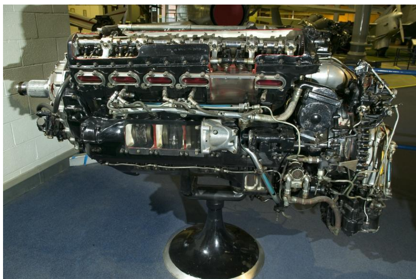
Fig. 1. Merlin 45 aeroplane engine, made by Rolls-Royce Ltd, Crewe, c.1941. From Science Museum Group, Merlin 45 Aeroplane Engine . Accessed: Apr. 24, 2025. [Online] Available: https://collection.sciencemuseumgroup.org.uk/objects/co8404794/merlin-45-aeroplane-engine . Licenced under CC BY-NC-SA 4.0 .
