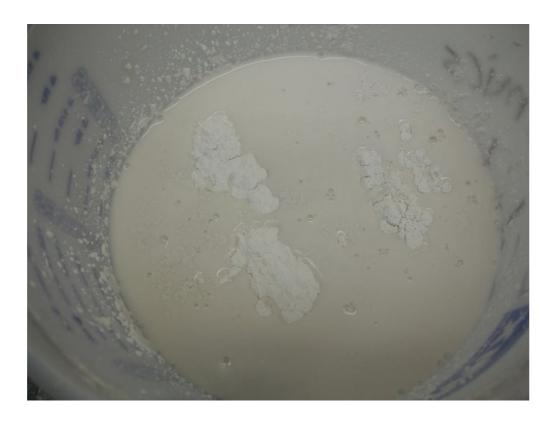
the absorbed plaster. Let the plaster sit for 2-5 minutes before stirring, this wait time ensures the plaster has fully absorbed the water and makes the plaster harder.
