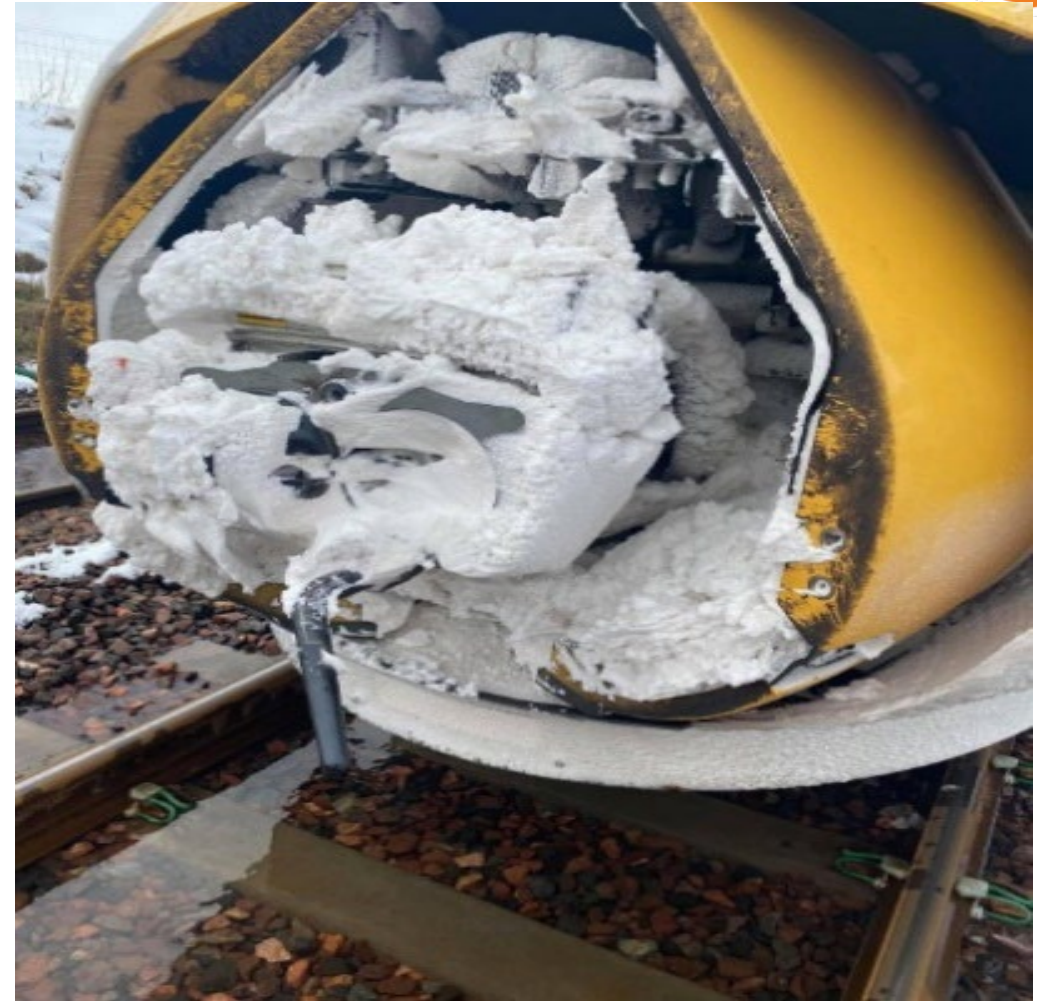
Frozen Coupler on an Intercity Express Passenger Train (IEP). Source: Mark Molyneux RDG
