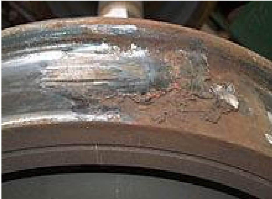
A damaged wheel caused by sliding on the rail head. Source: AWG. 2019.
