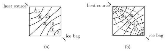
Figure 15: Temperature contours and heat flow lines for a metal plate
