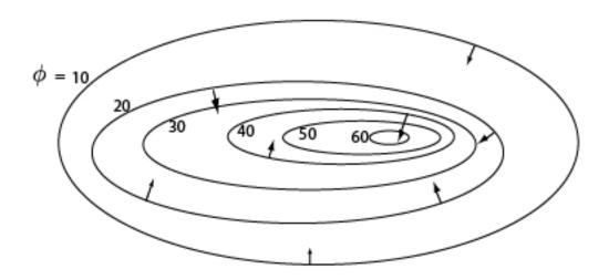
**Figure 16:** Grad  $\phi$  and the steepest ascent direction for a hill
